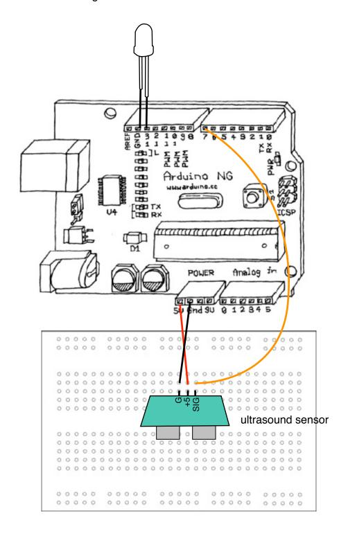
// Use an ultrasound sensor to turn an LED on. Sensor sends a wave out and then listens for it to bounce back. Stand at different distances from the sensor until you trigger the LED to turn on.
