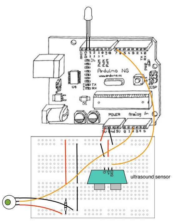
// Send a wave out with an ultrasound sensor; Use a potentiometer to turn on an LED at a particular distance from the sensor.
